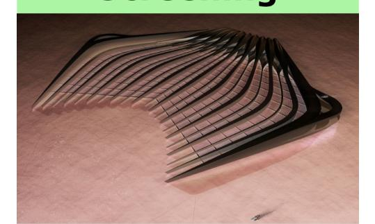
Marcella Hansch's platform consists of various canal systems that look like a water flows comb. The through the chambers, is calmed down and plastic with a lower density than water can be skimmed off.
